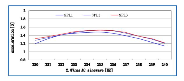
Note) The resonant frequency is normally distributed and controlled so as to be near 235Hz.
