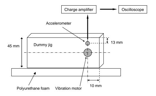
■ Specification of the dummy Jig
