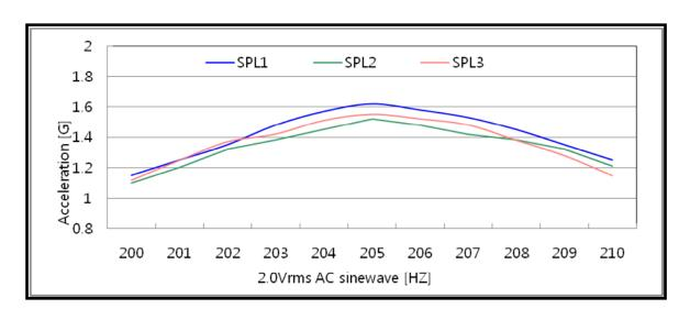
Note) The resonant frequency is normally distributed and controlled so as to be near 205Hz.
