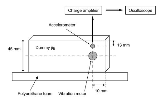
■ Specification of the dummy Jig
